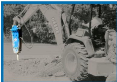
OP small hammers are suitable for use with mini excavators, skid steer loaders and tractor loader backhoes. Typical applications include demolition, excavation and trenching. Customized upper mounting brackets(UMBs) and quick coupler systems are available for all Okada breakers.
