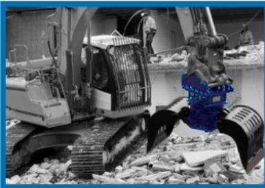
The Okada HD Rotating Grapple is engineered for efficiency and strength, handling a wide range of tasks including material handling, demolition, sorting, debris clearing, site preparation, and loading or unloading—delivering reliable performance through its durable construction and advanced functionality.
