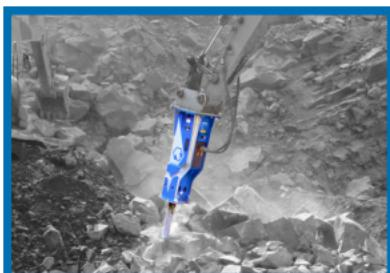
The internal control valve system equates to faster speeds and higher impact energy while still allowing the breaker to operate at cooler temperatures. The Anti-Blank Firing System is available on ORV2500H through ORV12000H models, helping protect internal components from damage by preventing firing when the tool is not engaged with material.
