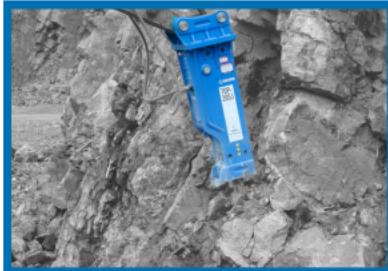
TOP medium to large hammers feature a simplified design with fewer components, reducing issues. Matched to the right carrier, TOP breakers use nitrogen cushioning to minimize vibration, lowering operator fatigue and equipment wear. All models come in box-type housings.
