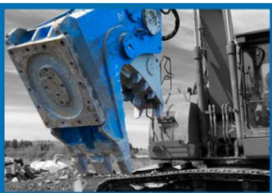
Secondary breaking crushers were developed as a result of a growing need to reduce disposal volume and recycle concrete waste created during concrete building demolition. The flat, wide jaw design and an internal speed valve make it possible to grab and crush large sections of concrete quickly.
