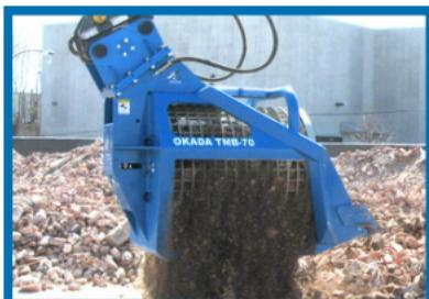
The compact, robust frame design makes the TMB lightweight and easy to handle. Each unit comes equipped with an integrated control valve to regulate hydraulic flow and pressure, eliminating the need for additional plumbing on the carrier excavator.
